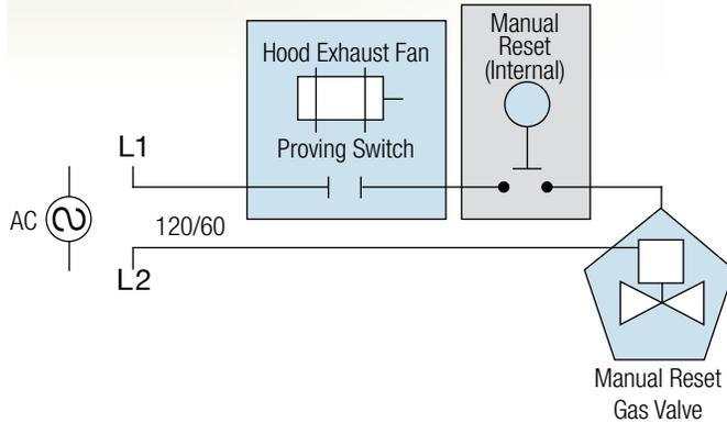
Under the NFPA (54) Code 10.3.5.1 & 10.3.5.2 (2002), ventilating hoods and exhaust systems shall be permitted to vent gas-fired equipment installed in commercial applications. However, certain requirements must be met, including:
