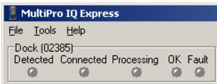
When a detector is placed in the dock, the indicator will change to reflect the new status. Status changes are also be shown on the dock's LCD.
