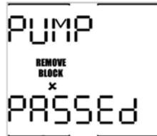
If the instrument is unable to detect the vacuum resulting from the pump blockage, the test will fail and you will be directed to remove the pump.
