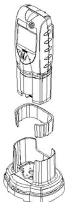
charger, and with the guide pins facing down towards the charger as shown in the illustration at right.
