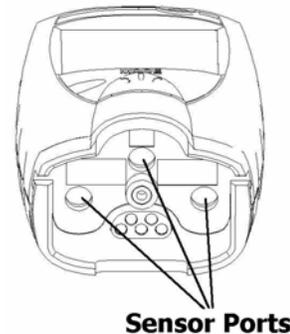
In diffusion mode, the atmosphere being measured reaches the sensors by diffusing through vents in the bottom of the instrument. Normal air movements are enough to carry the sample to the sensors. The sensors react quickly to changes in the concentrations of the gases being measured. Diffusion-style operation monitors only the atmosphere that immediately surrounds the detector.
