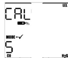
2. Press the MODE button before the end of the 5-second countdown and **continue to hold the MODE button**. As in the
