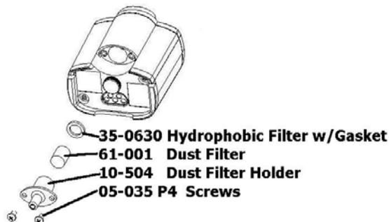
4. The hydrophobic filter is located beneath the inlet port in the pump housing. Use a small screwdriver or other object to punch through the filter and remove it. The gasket that sits between the inlet port and the filter should come out with the filter.
