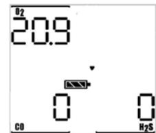
**⚠WARNING:** Always verify that all sensors present in the instrument are shown on the current gas readings screen whenever the MultiPro™ is turned on. Failure to verify sensor presence prior to use in a hazardous location may result in serious injury or death.
