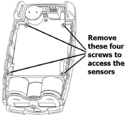
Remove these four screws to access the sensors
