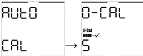
2. Press the MODE button before the end of the 5-second countdown to begin the fresh air/zero calibration. The fresh air/zero calibration has been initiated when the MultiPro alternates between the following two screens:
