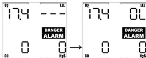
**⚠WARNING** A combustible sensor overrange alarm indicates a potentially explosive atmosphere. Failure to leave the area immediately may result in serious injury or death!
