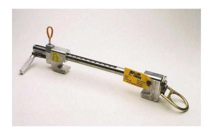
Miller Shadow Beam Anchors connect horizontally to a wide range of I and H beam flanges from 4 inches (100mm) to 24 inches (610mm) wide and up to 2-1/2 inches thick. The fixed unit (Model 8815) is designed to be tightened horizontally or vertically, firmly gripping the beam or column to provide a temporary or permanent anchorage attachment.
