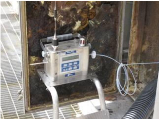
AreaRAE monitors were operating 17 hours a day and were calibrated each week. The wireless monitors were placed on a catwalk 40-foot (12m) high with 20 feet (6m) of tubing running from the units to the chamber being serviced. Typically, two chambers were serviced at any given time. The sample tube was placed at worker breathing height using a simple stand.
